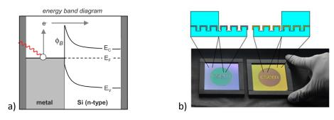
Figure 1: a) Band diagram for plasmonically driven hot electron injection over a Schottky barrier ( $\varphi_B$ ). Source: M.W. Knight <sup>[5]</sup>. b) Large area plasmonic structures developed and manufactured at CSEM.
