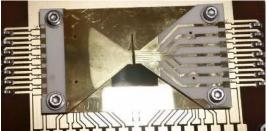
In a current project funded by the SNI, we have developed an experimental setup in which a laser-cooled trapped Ca<sup>+</sup> ion is coupled to a charged Ag2Ga nanowire (see figure).
