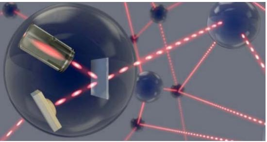
At each node point in the quantum network, the aim is to link a photon source with a quantum memory. The information is then transmitted using entangled photons. (Image: Department of Physics, University of Basel)
