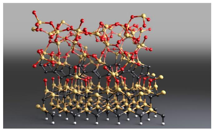
The oxidation process of silicon carbide forms defects: At the interface between silicon carbide (periodic black-yellow atoms) and the insulating silicon dioxide (red-yellow atoms), irregular clusters of carbon rings (irregular black structures embedded in red and yellow atoms) occur. These are bound within the crystal lattice and disturb the current flow. (Image: Departement of Physics, University of Basel)
