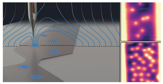
The Poggio team succeeded in imaging vortices in MoSi for the first time using a newly developed, highly sensitive superconducting quantum interference device at the end of a tiny scanning probe. (Image: L. Ceccarelli, Department of Physics, University of Basel)
