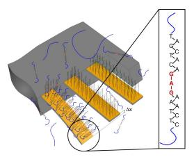
The cantilever on the left bears the recognition sequence for the target mutation. If this is present in the sample being tested, the corresponding segment of RNA binds to the cantilever, causing the latter to bend. This can be measured, providing clear evidence that the genetic change is present.
