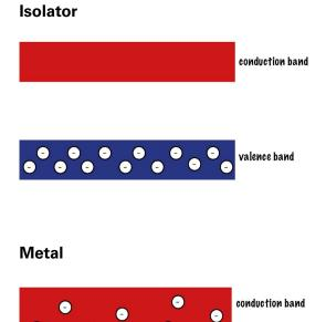
In an insulator, the valence and conduction bands are separated by an energy gap. The energy gap represents the amount of energy that must be supplied to "excite" an electron from the valence band into the conduction band. There is no energy gap in a metal that conducts electricity. As a results, freely mobile electrons are always available and current can flow without the need for thermal excitation.
