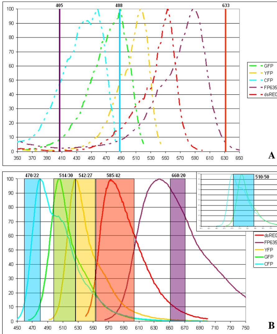
**Fig. 1:** Excitation (A) and emission (B) spectra for the different fluorescent proteins, the box in the upper right corner of B shows the emission spectra of CFP and GFP/GFPuv that are detected using a 510/50 bandpass filter
