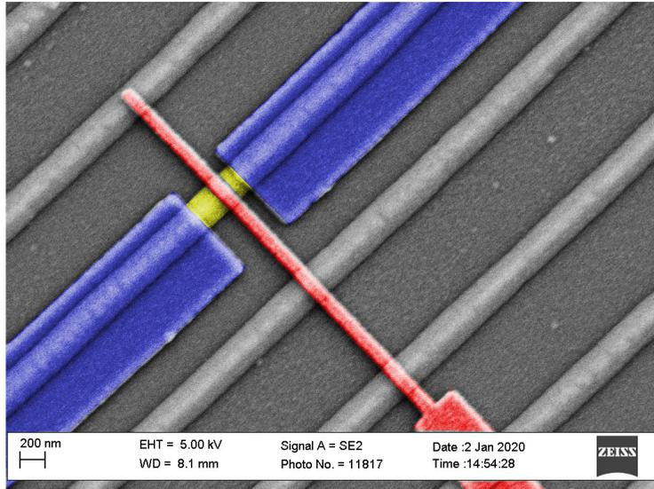
**Figure 7:** False-colored SEM image of the arrangement. With the 140 nm thick wires (yellow) which are contacted from the side by Ti/Au (blue). The contacts are separated by 450 nm. Above the HfO<sub>2</sub> dielectric layer 90 nm wide gates (red) are deposited by EBL to apply a voltage in order to pinch-off the wire.
