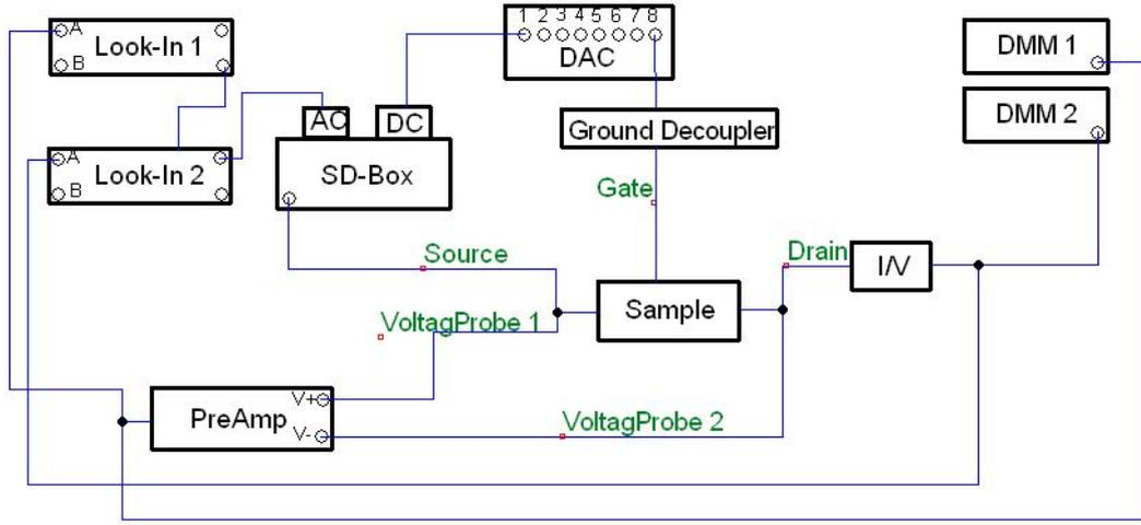
**Figure 8:** A schematic of the used measurement set up. The lock-in, DMM and the DAC were connected to a computer to read out the measurements and to set parameters, as for example the voltage applied to the source drain.
