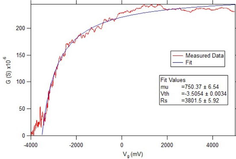
**Figure 12:** A representative measurement result of the conductance, while reducing the gate voltage till the wire is pinched. By using Equation 10 the mobility is extracted. For the capacitance  $C$  it is assumed that we have a plate capacitor and  $L$  is the width of the used gate to pinch the wire.  $R_s$  is the resistance extracted by the fit for the measurement set up and  $\mu$  is the mobility which is here about  $750 \text{ cm}^2/\text{Vs}$ .
