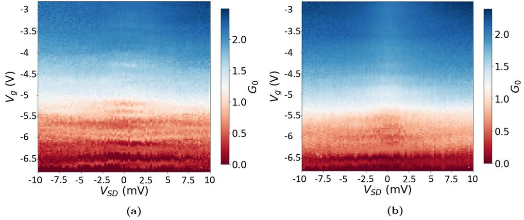
**Figure 15:** Bias spectroscopy of a 220 nm thick wire, of the  $\text{Al}_2\text{O}_3$  sample. The color scale on the right is in units of  $2e^2/h$ . The same measurement was done at zero field (a) and at 8 T magnetic field (b). The magnetic field is applied perpendicular to the sample plane. There is no significant difference between those two measurements. These results indicate that there is no ballistic transport due to the absence of diamonds.
