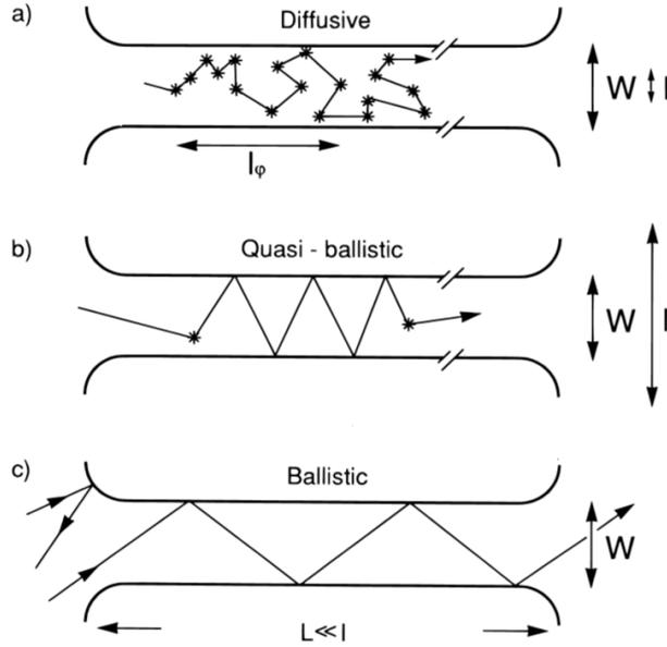
**Figure 5:** Illustration of the different transports. **(a)** The diffusive transport for  $L, W \gg l$ , **(b)** quasi-ballistic transport for  $W < l < L$ , and **(c)** ballistic transport for  $W, L \ll l$ . Figure taken from [42].
