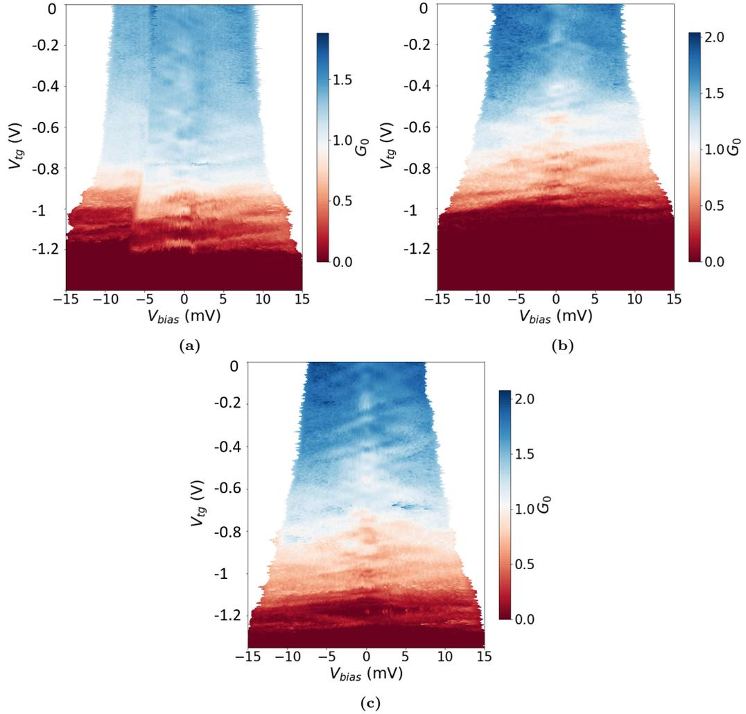
**Figure 17:** Bias spectroscopy measurements for different NW renormalized. (a) Measurement result of the 150 layer sample measuring a 35 nm wire of distance 300 nm and a 60 nm gate. In the data there can be seen a charge switcher. (b) the 200 layer sample measuring a 50 nm wire of distance 200 nm and a 60 nm gate, and (c) the 200 layer sample measuring a 35 nm wire of distance 200 nm and a gate above the full length of the wire. Here in (c) the diamonds can be seen the clearest.
