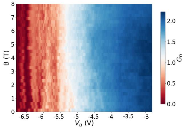
**Figure 16:** Zero bias conductance measurement of a 220 nm thick wire, of the  $\text{Al}_2\text{O}_3$  sample, while varying the magnetic field and the top gate. The magnetic field is applied perpendicular to the sample plane. The color scale on the right is in units of  $2e^2/h$ . Also, this measurement indicates that there is no ballistic transport.
