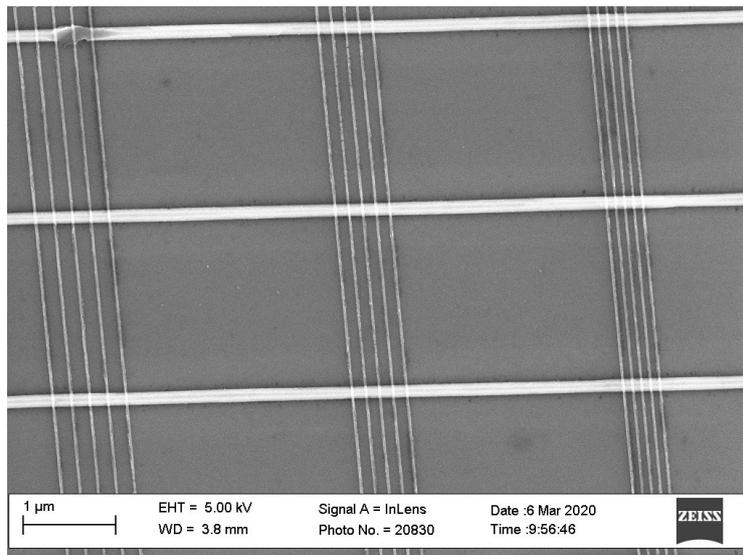
**Figure 19:** SEM image taken with the InLens. One can see that the lift-off did work, and the gates are separated also on the wire. With still occasional breaks in the wire, which indicated that we do not have the proper dose, yet.
