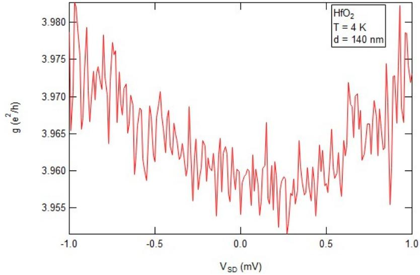
**Figure 9:** A representative measurement of the conductance, while sweeping the source drain voltage from  $-1$  to  $1$  mV of a  $140$  nm thick NW.
