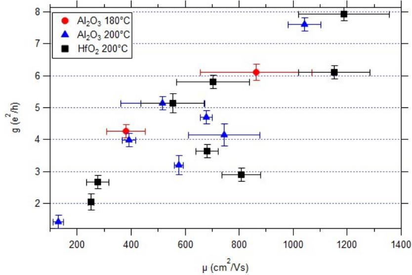
**Figure 13:** The conductance is plotted against the extracted mobility. One can see as expected from Equation 7, the linear dependence of the mobility to the conductance.
