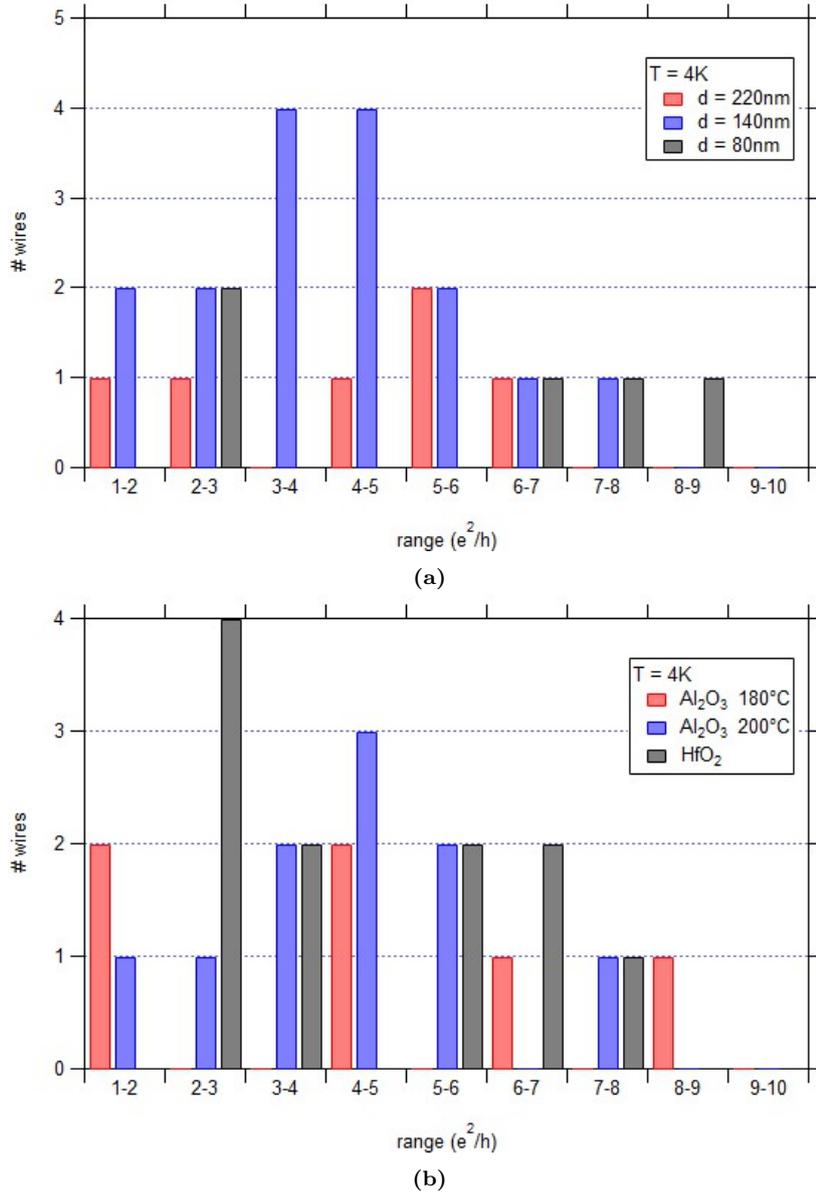
**Figure 10:** The histogram shows the number of wires conducting in a certain range. The results are separated by the defined NW width's **(a)**, respectively **(b)** by the oxide.
