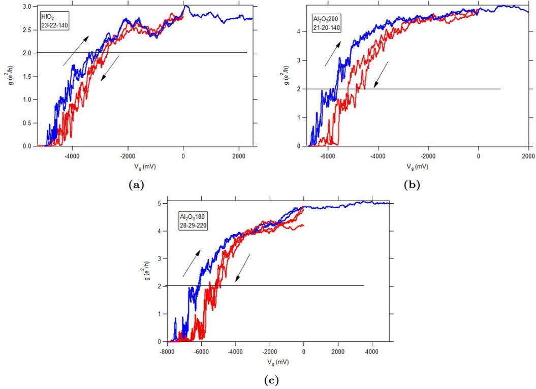
**Figure 14:** Representative pinch-off curves for the  $\text{HfO}_2$  (a), the  $\text{AlO}_2$   $200^\circ\text{C}$  (b), and the  $\text{AlO}_2$   $180^\circ\text{C}$  (c) samples. The arrows indicate the direction of sweep, the red curves are the sweeps from positive to negative voltage and the blue ones are vice versa. The black horizontal line helps to see the plateau around  $2e^2/h$ , which might be due to quantized conductance.
