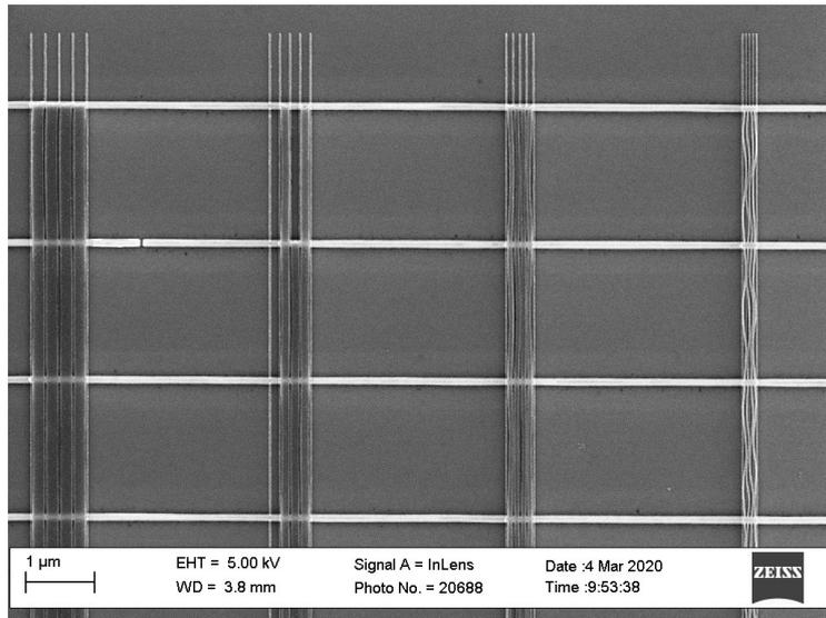
**Figure 18:** SEM image taken with the InLens. One can see that the lift-off did not work properly, due to too much exposure on the InAs wires, where the resist is assumed to be thinner than above the SiO<sub>2</sub> mask.
