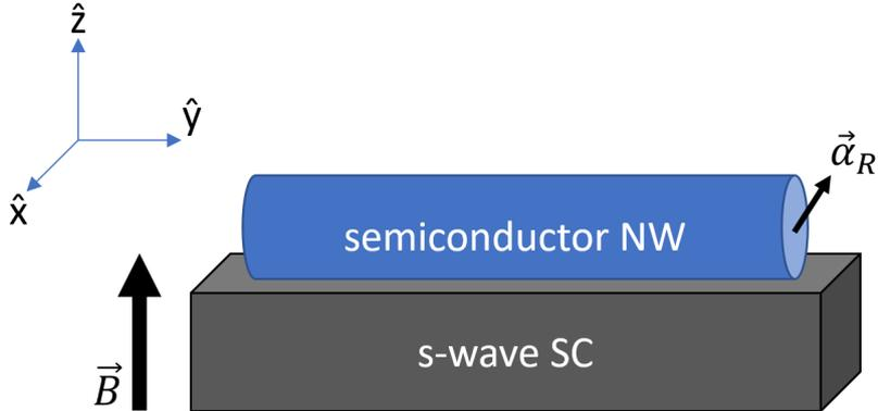
**Figure 2:** An illustration of a possible system, which in theory gives rise to unpaired MF. A semiconductor nanowire with strong Rashba spin-orbit coupling is placed in proximity to a s-wave superconducting material. Perpendicular to the resulting effective magnetic field  $B_{SO}$ , a magnetic field  $B$  is applied, here in the direction of  $z$ . Figure inspired by [28].
