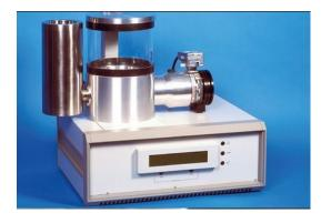
This is why the NI Lab decided to invest in an **EMS 775 Turbo Freeze Dryer**. It operates at temperatures down to -140°C and employs a Turbomolecular pumping unit, backed by a Rotary Vacuum pump. The lower temperatures are achieved by using a Liquid Nitrogen fed Cold Stage.
