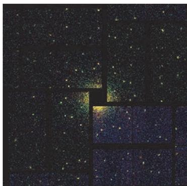
Fig. 1: Diffraction pattern from 2D crystals of bacteriorhodopsin obtained with a femtosecond XFEL pulse. The crystal suspension was prepared on a silicon nitride membrane support [3].
