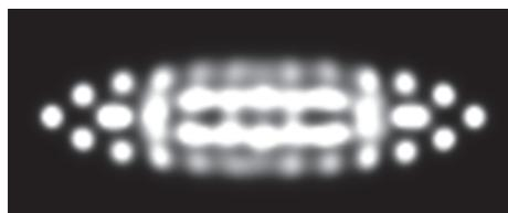
Fig. 2: Simulated picture of a Coulomb crystal of 50  $\text{Ca}^+$  ions formed in the chip trap at a temperature of 30 mK.
