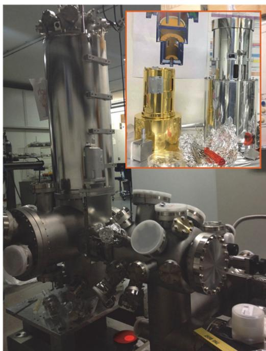
*Fig. 1: Current status of the new LT-AFM, shown from left to right: analysis chamber with the housing for the microscope head and the cryostats on top and preparation chamber. Not visible here is the manipulator which was recently mounted to the right site of the preparation chamber. Inset showing the outer cryostat for liquid nitrogen (right) and inner cryostat for liquid helium (left).*
