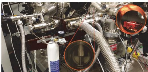
Fig. 3: Setup for the graphene preparation at PEARL. A long nozzle (600 mm) with a z-drive (300 mm) – bellow visible in the image centre – is mounted to the preparation chamber. Valves at the rear of the nozzle allow for control of the gas flow. The upper right inset shows the approached nozzle. The inset in the lower middle is showing the guide that stabilizes the nozzle. Ion pump and z-drive were provided by R. Stania and T. Greber, University of Zürich.
