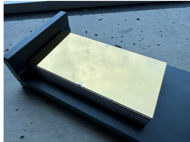
Fig. 1: Picture of a full GaAs:Cr module ( 8 \times 4 \text{ cm}^2 ) mounted on eight JUNGFRUA readout chips.
