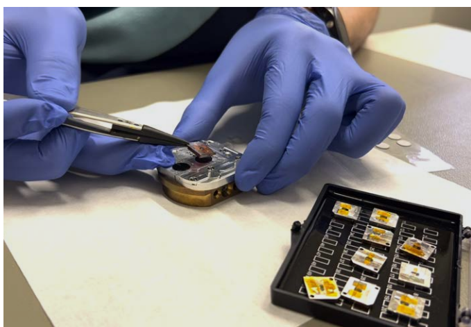
The developed method will help the researchers place electrical contacts on the tip of an atomic force microscope cantilever and thus produce highly sensitive probes for studying electric and magnetic fields.
