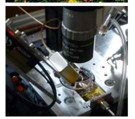
Using nitrogen-vacancy (NV) centers in diamonds, it's possible to detect the magnetic fields of tiny magnetic particles in liquids.
