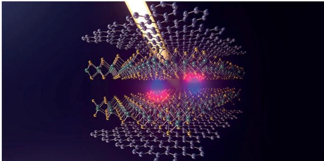
Schematic illustration of the electron-hole pairs (electron: pink, hole: blue), which are formed by absorption of light in the two-layer molybdenum disulfide layer. Credit: Nadine Leisgang and Lorenzo Ceccarelli, Department of Physics, University of Basel
