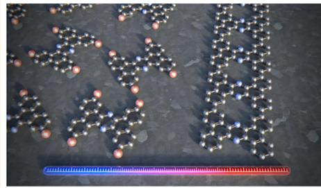
IMAGE: The individual building blocks are heated on a silver surface in order to synthesize a porous graphene ribbon that exhibits semiconducting properties and a ladder-like structure. In each rung of...
