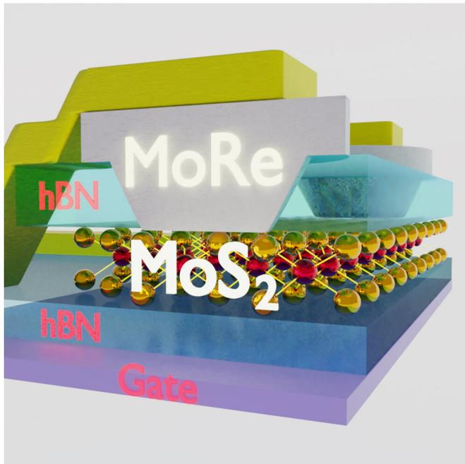
The monolayer of molybdenum disulfide ( $\text{MoS}_2$ ) is sandwiched between two protective layers of boron nitride (hBN), with molybdenum rhenium (MoRe) contacts extending through the upper one. A layer of graphene (gate) is used for electrical control. Credit: Mehdi Ramezani, Swiss Nanoscience Institute, University of Basel
