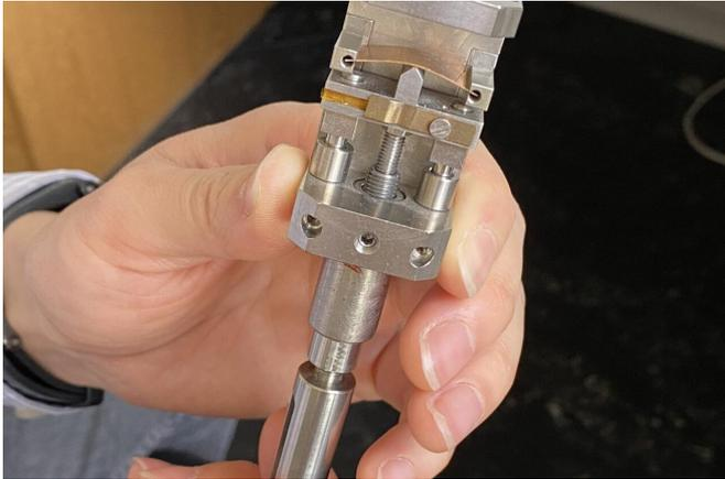
Force from below causes the component to bend. This elongates the embedded graphene layer and changes its electronic properties. Credit: Swiss Nanoscience Institute, University of Basel
