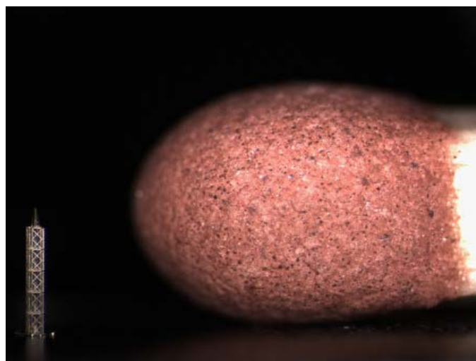
Photograph of the refractive X-ray lens (left bottom corner) compared to a head of matchstick. Such 3D printed microstructure was combined with a Fresnel zone plate to realize the apochromatic X-ray optics (Photo: Paul Scherrer Institut / Umut T. Sanli and Joan Vila-Comamala).
