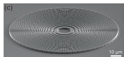
Fig. 1: a) Achromat X-ray focusing can be realized by the combination of a refractive and diffractive lens. b) Refractive X-ray lens fabricated by two-photon polymerization 3D printing. c) Diffractive X-ray lens fabricated by electron-beam lithography and nickel electroplating.
