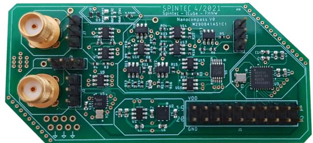
Fig. 6: Control and signal processing electronics.
