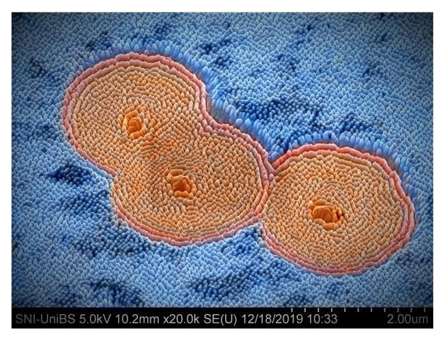
This image is a top-view of a single-crystal rhodium imaged by a Hitachi S4800. The exposure of the Rh surface to Ar+ leads to the appearance of ripples that propagate outwards, eventually leading to coalescence.
