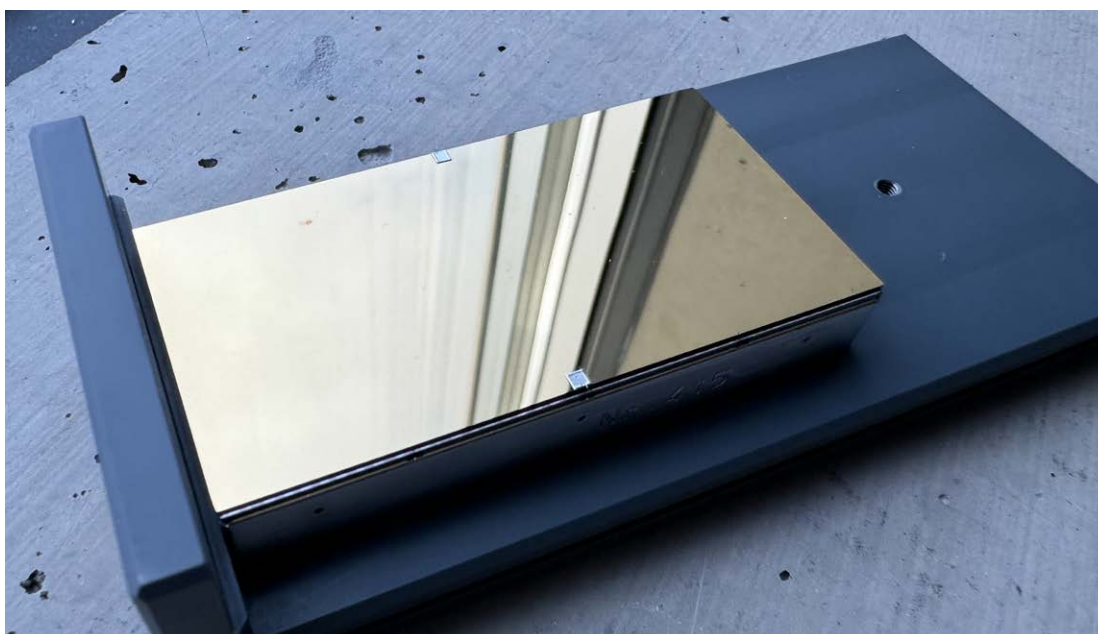
Researchers working on the Nano-Argovia Project HiZfEM plan to improve image quality in transmission electron microscopy by using new detector modules such as this one made of chromium-doped gallium arsenide (8 x 4 cm 2 ).
